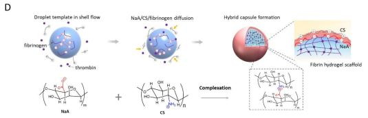
Illustration of synthesizing composite capsules in microfluidic device
