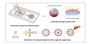
One-step synthesis of composite hydrogel capsules (CHCs) that allow to engineer hiPSC-derived liver organoids in an oil-free droplet microfluidic system.
