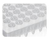
The edge of the wells is protruding to prevent cross-contamination and to facilitate sealing
