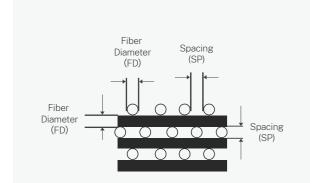
Average fiber diameter: 500  $\mu m$  (FD); average spacing of fiber column: 260  $\mu m$  (SP)
